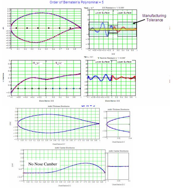
Figure 3: RAE2822 Geometry Characteristics
