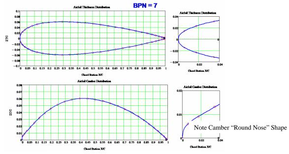
Fig. 5. NACA6412 Camber and thickness distribution
