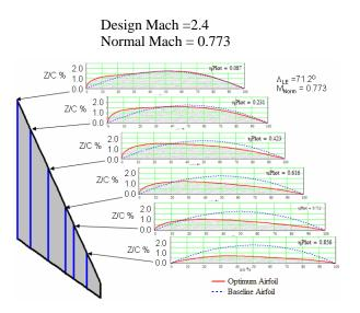
Fig. 7. Subsonic Leading Edge Supersonic Wing Design
