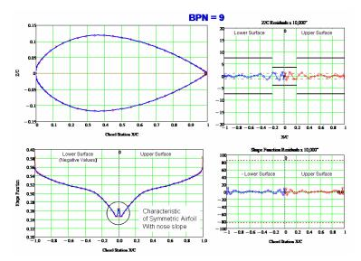
Fig. 6. Symmetric Round Nose Airfoil with additional Finite Nose Slope term The "hook" in the shape function near the airfoil nose is indicative of the presence of a finite nose slope term.
