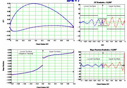
Figure 4. NACA 6412 Airfoil and Shape Function
