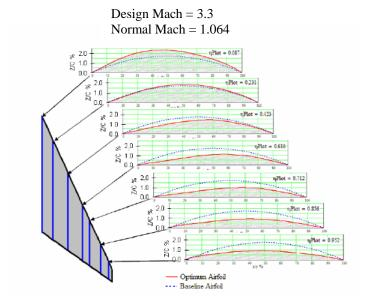
Fig. 8. Supersonic Leading Edge Supersonic Wing Design
