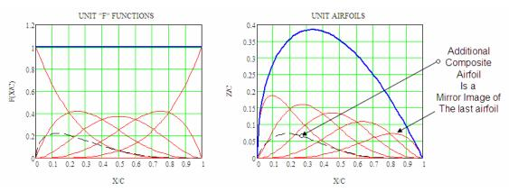
Fig. 2. BPO4 Composite Shape functions and Composite Airfoils With Additional Sharp Nose Composite Airfoil.
