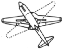
Blohm and Voss (Vogt) Oblique Wing Fighter Concept (1944)
