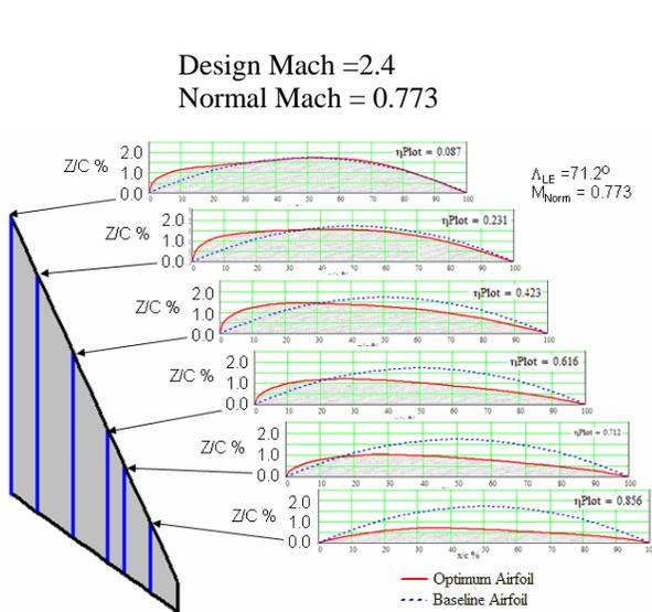
Fig. 7. Subsonic Leading Edge Supersonic Wing Design
