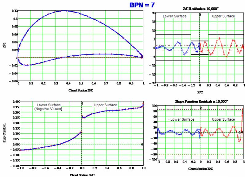
Figure 4. NACA 6412 Airfoil and Shape Function
