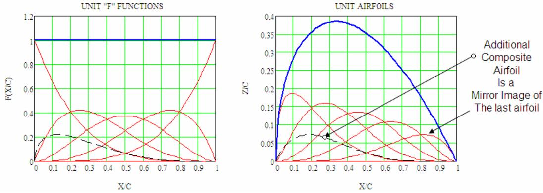
Fig. 2. BPO4 Composite Shape functions and Composite Airfoils With Additional Sharp Nose Composite Airfoil.
