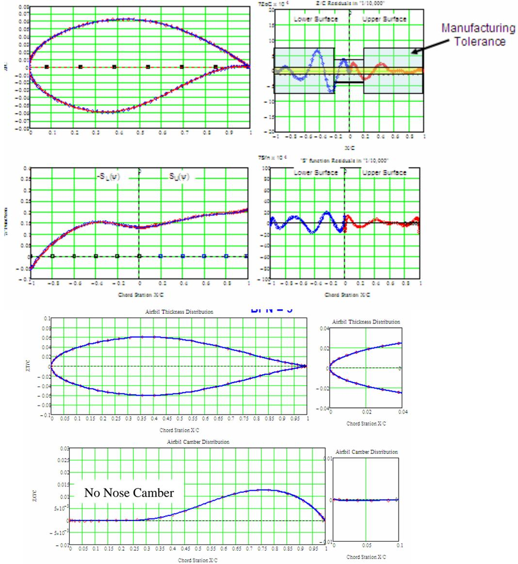
Figure 3: RAE2822 Geometry Characteristics
