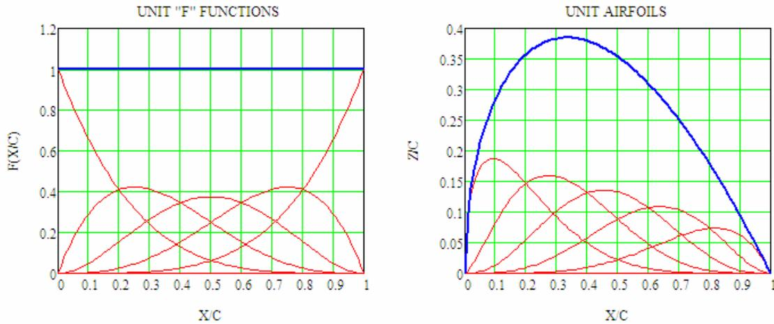
Fig. 1. Composite Shape Functions and Composite Airfoils for a BPO = 4 Unit Shape function Airfoil
