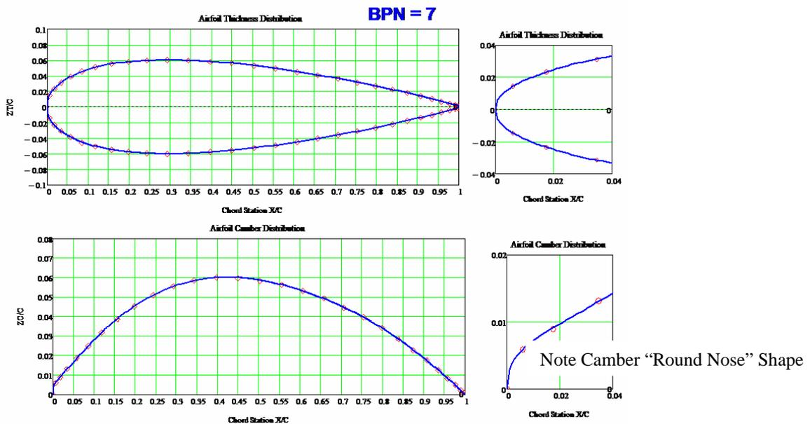
Fig. 5. NACA6412 Camber and thickness distribution
