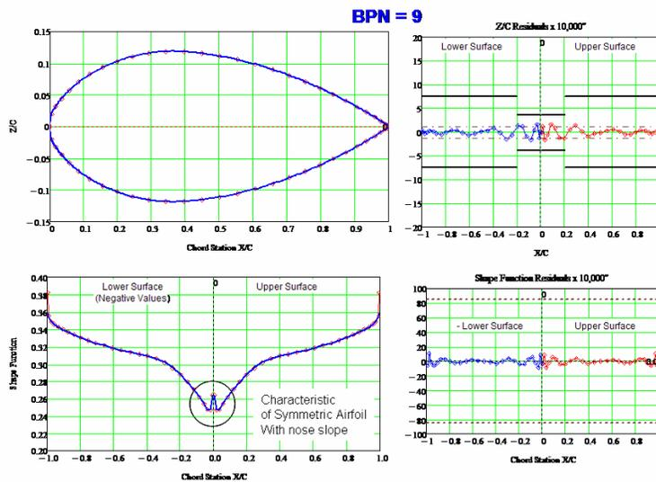
Fig. 6. Symmetric Round Nose Airfoil with additional Finite Nose Slope term
